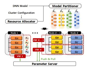
Fig. 4. The architecture of the proposed cluster system
