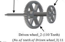
$Gear Ratio = \frac{(NO.0)}{(No.of teeth of Driven wheel_2) 110} = \frac{1}{10}$
