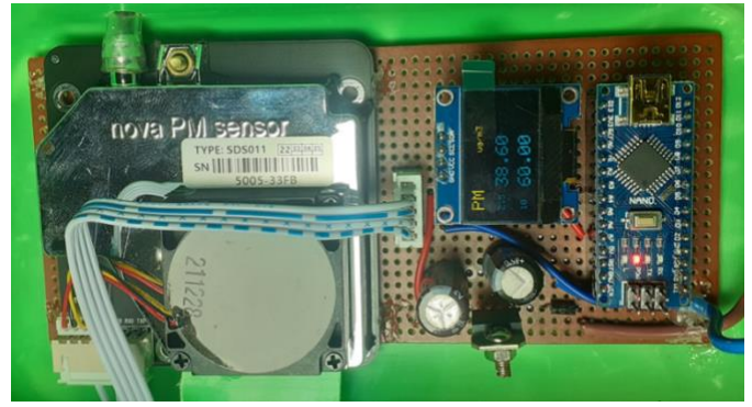
Fig. 6. PM monitoring unit with SDS011 sensor, OLED display with arduino nano
