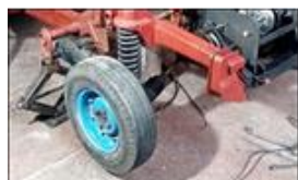
Fig. 11. Tire lifted to get the neutral condition.
