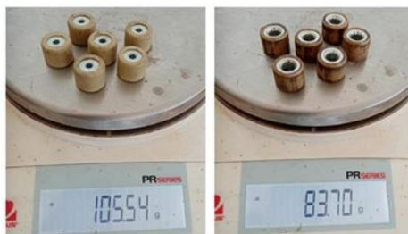
Fig. 13. Two types of the Roller weights
